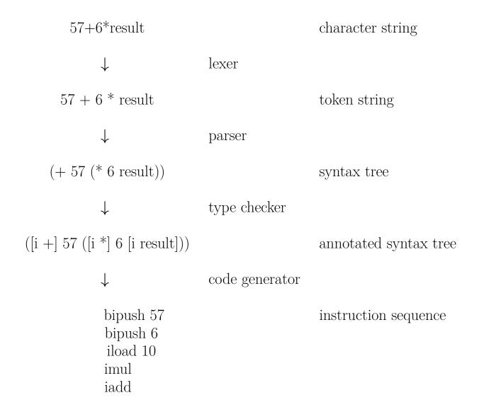
Compilation phases from Java source code to JVM assembly code
